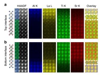
**Fig. 2** Atomic structural characterization of the two interfaces in the LAO// STO/LAO heterostructure. **a, b** show the energy-dispersive X-ray spectroscopic (EDS) mappings of the top and bottom interfaces, respectively. From left to right: schematic structures, high-angle annular dark-field image, Al K, La L, Ti K, and Sr K EDS integrated signal maps, and the combined elemental maps of all cations
